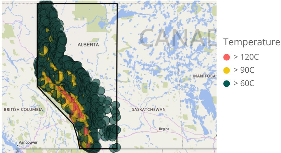
Figure 2. Inactive O&G wells potentially suitable for geothermal energy production
