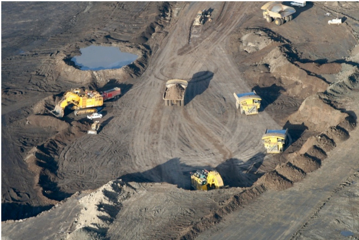
Figure 3: Nearly 2,000 kg of oil sands ore are mined for each barrel of oil produced
