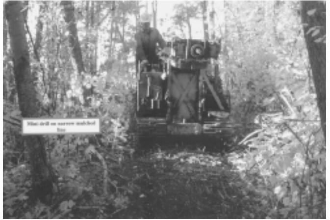
Small seismic shot hole drills can operate on narrow source lines.
