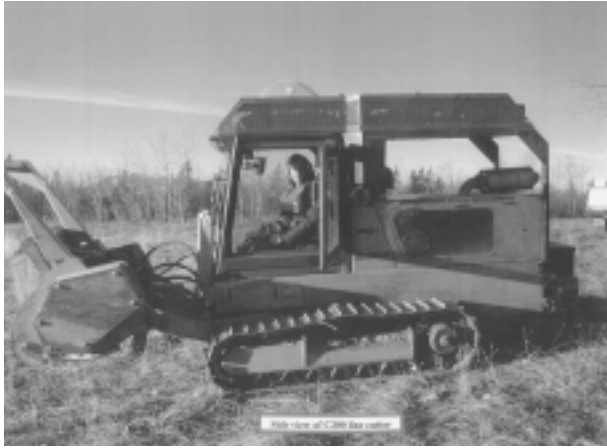
A small mulcher can be used to create meandering source lines less than 2 metres wide.
