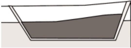
Sump used for collecting drilling waste.
