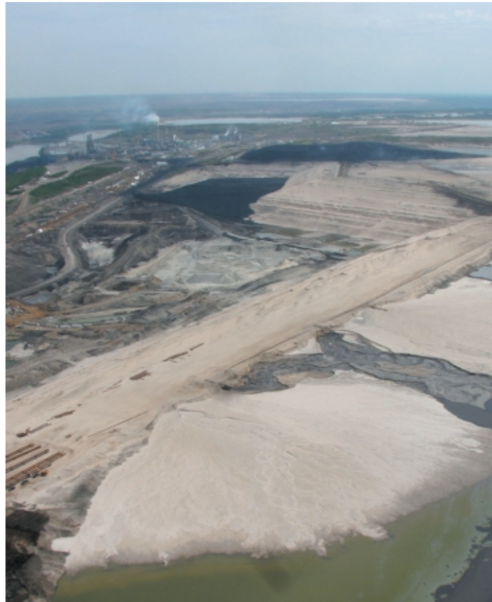
▲ Tailings ponds, mining operations and production facilities comprise the landscape of oil sands operations, examples of which include the Suncor operation along the Athabasca River (bottom) and the Syncrude upgrader near Highway 63 (top).
