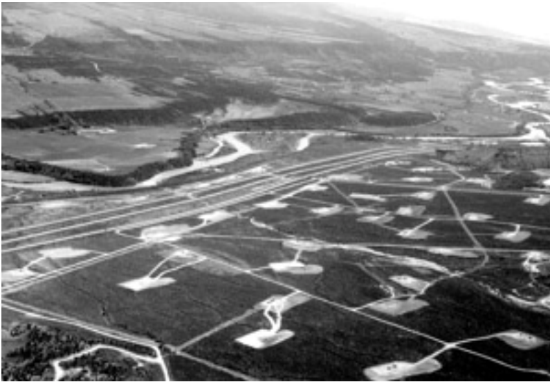
Figure 3.2 Densely spaced coalbed methane wells in Colorado with access roads, drill sites and containment ponds
