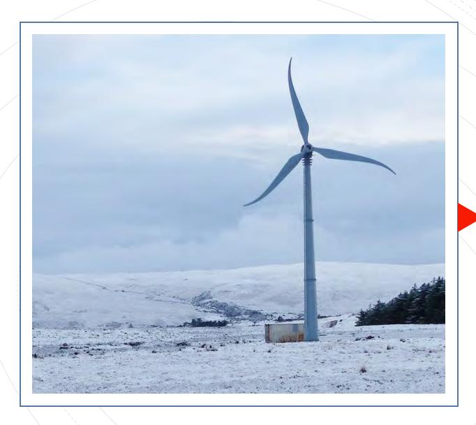
10 Self-Erecting 32 Meter tall 90 kW Craneless Wind Turbine Towers being considered
