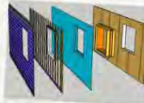
Built-up structurally insulated panel (SIP)
