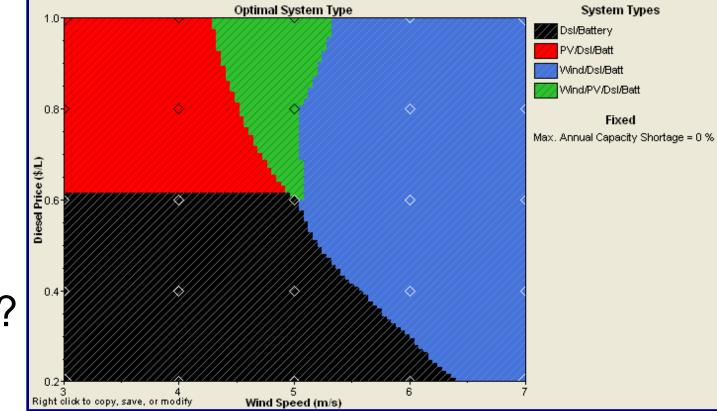
Combining sensitivity and optimization identifies design thresholds. e.g. minimum fuel price for cost-effective PV
