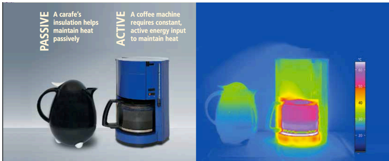
Figure 7. Passive vs. active approaches to climate control
