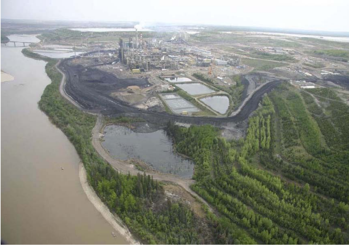
Figure 22: The long-term viability of tailings dykes will remain an ongoing concern long after operations cease. Dyke failures could release unstable materials into the Athabasca River, with catastrophic effects on the aquatic ecosystem.
